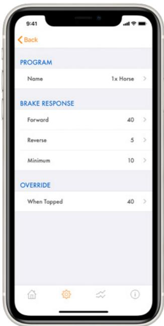
2. When driving at 25kmh apply **light pressure** and assess trailers braking response.
