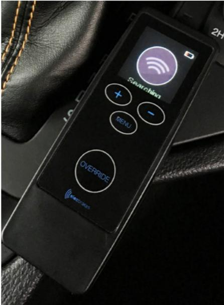
3. When connected to an ELBC 2000 the screen will display a tick and active program will be displayed.
