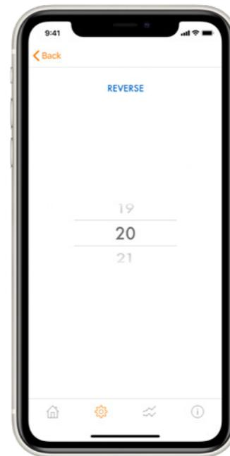
Elecbreaks recommend adjustments in 5-point increments initially. Finer adjustments can be made to gain a smooth braking response.
