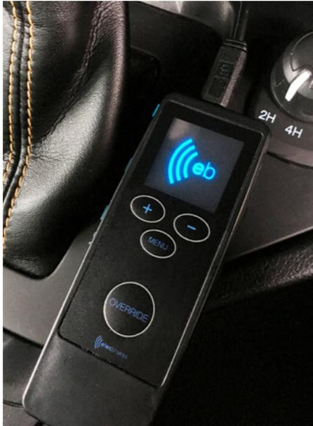
2. Once completing its start up the remote will automatically start to search for a device. The screen will display as searching.
